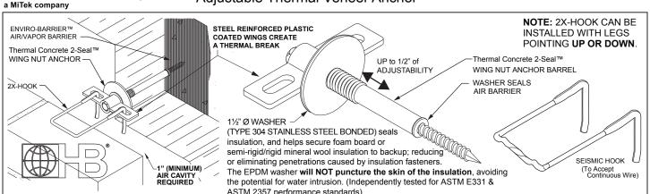
Hohmann & Barnard's 2X-Hook has been tested and designed to withstand over 200-lbf, in tension or compression, at maximum allowed offset (TMS 402/602-16 12.2.2.5.5.4) of 11/4" (disengagement of the pintle from the veneer anchor). These results exceed BIA recommendations and the capabilities of standard "round wire" hooks/pintles by over 100%, while maintaining the ASTM A1064/1064M wire specification.
